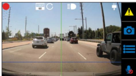
Align front edge of the hood below the blue line (20% max from bottom)
